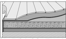
Engineered Wood Flooring on Duo-Protect / Mineral screed
