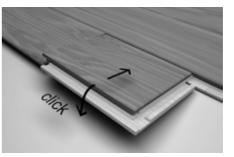
Patented click-mechanism The patented AUTOMATIC-CLICK mechanism with its long and end edge locking system makes quick, trouble-free installation possible without glue.
