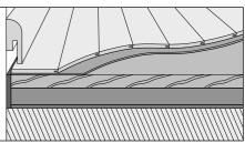
Engineered Wood Flooring on Uno-Protect / Hardwood planks
