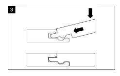
Fig. 2 + 3: Begin the second row on the left side by clicking the longitudinal tongue of the first board into the groove of the first row. To do so, insert the tongue into the groove at an angle of approx. 25° and lower the board. As it is lowered the board snaps into place tightly giving you a press fit.
