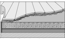
Engineered Wood Flooring, all-over adhesion
