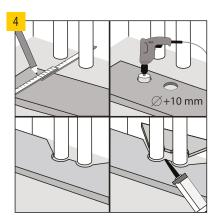
Act similarly in the case of a bigger number heating system pipes. The cut panel elements must be joined with the assembly adhesive for plastic elements.
