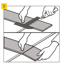
For additional cutting of floor panels, use a sharp knife, cut the top layer, then break the panel dynamically by leaning it on the edge. The floor panels may also be easily cut using an electric saw.
