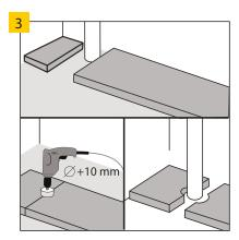
In the case of vertical pipes embedded in the substrate, leave free space around the pipes. Holes for the pipes must be drilled with a drill bit with a diameter that is bigger than the pipe diameter by 15 mm.
