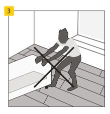
The movement of heavy objects along the floor is not allowed. They must be moved only after they are lifted.
